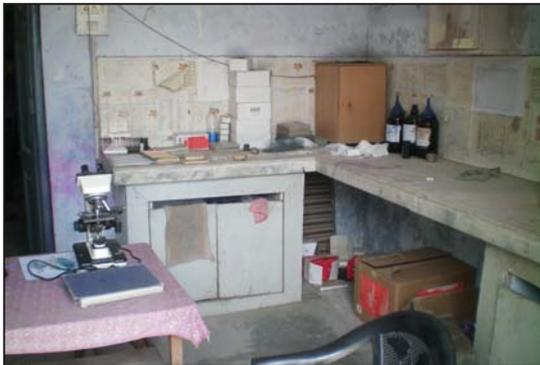
Photo 5: Flammables, acids, and bases are all stored separately from each other.
